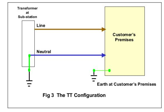
Previously this represented the arrangement for overhead line supplies, as these did not have a separate earth conductor from the substation. Today this arrangement is still normally used where a TN-C-S customer's earth terminal cannot be provided, for example when the property incorporates a swimming pool or a caravan site.
