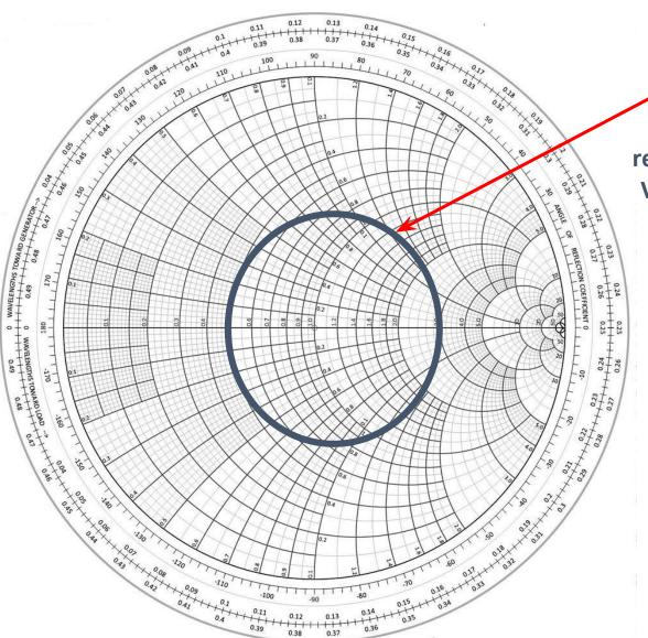
Any circle centred around the normalised impedance point represents a constant VSWR. The bold blue line passes through  $25\Omega$  and  $100\Omega$  resistance points, so any point on that circle is 2.0:1 VSWR
