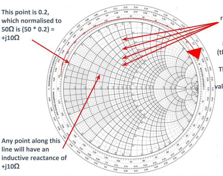
These dark lines represent a range of impedances which have constant inductive reactance (the "imaginary" part of the impedance). The scale around the outside gives the value of the reactance relative to the normalised impedance.
