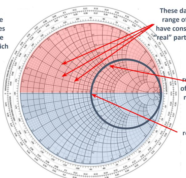
These dark lines represent a range of impedances which have constant resistance (the "real" part of the impedance).
