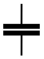
It varies with frequency. With a DC voltage applied there is no current flow at all. If an AC voltage is applied, then the reactance is dependant upon the frequency.
