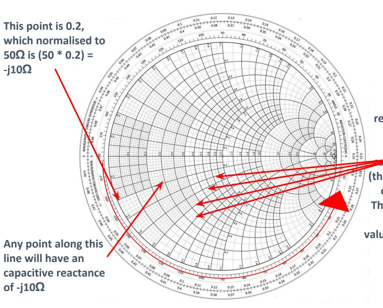
These dark lines represent a range of impedances which have constant pacitive reactance (the "imaginary" part of the impedance). The scale around the outside gives the value of the reactance relative to the normalised impedance.
